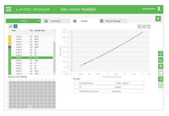
Figure 3: Illustration of the Results screen on the Lunatic. Reference samples (shown as yellow crosses) are used to create a standard curve and concomitant equation to calculate the concentration of protein samples (gray squares, red if selected).
