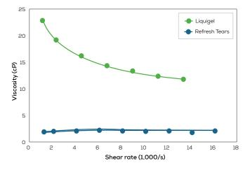
Figure 2: Viscosity measurement of Newtonian and non-Newtonian solutions.
